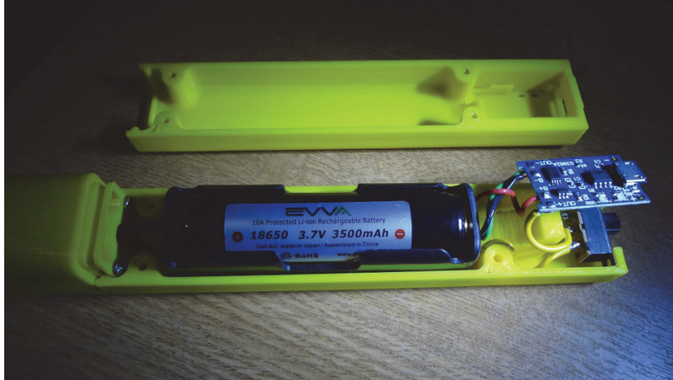
FIGURE 8 – All components mounted and wired
