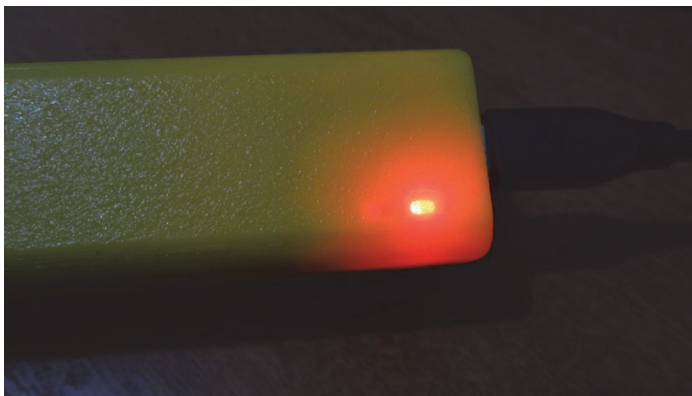
FIGURE 13 – The charging LEDs can be easily seen from outside
